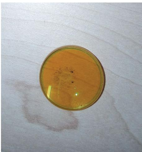
Dust spots burned into the lens will cause the beam not to focus correctly - news lens needed.
