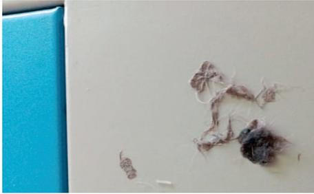
Actual cat hair removed from a tube, pipes and water flow sensor.
