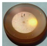
Same goes for mirrors and the lens. The mirror on the far left has a burn mark caused by dirt build-up, while the lens next to it is destroyed because the laser was run with dust on the lens.
