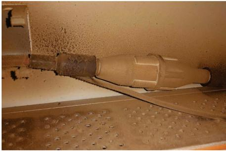
The high-voltage connector between the power supply and the tube **MUST** be kept dust-free & clean at all times.
