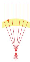
A speck of dirt will cause the lens to overheat and damage the coating on the lens.
